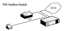
TUVM connects directly to a telephone instrument and fax machine via its FAX interface. This interface allows a fax machine to operate over its normal PSTN line or share access to the MICOM integrated network.
